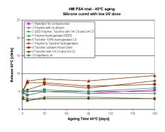
Graph 3 – Silicone cured at 240 ppm residual oxygen Various Hot-Melt PSAs on RC Silicone-Coated Release Liner
